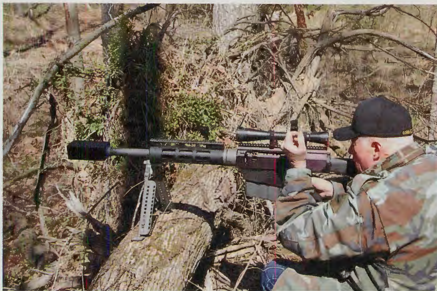
Johnston found that opening the bolt on the BA-50 was super smooth, thanks to its rollers. His shooting hand never leaves control of the pistol grip.
